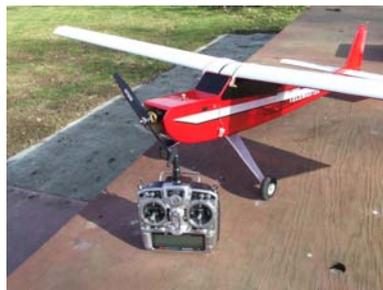
Telemaster Electric 73 inch AXI-2826-12, Jetti-40 amp controller, A123 4 cell 2300 mAh battery, AR7000 RX, JR X9303 TX
